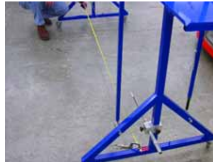
Extend tape to outside of opposite side of device.
