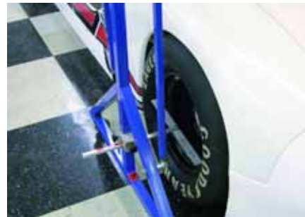
Front tread width is measured by viewing gauge on right side measuring arm.
