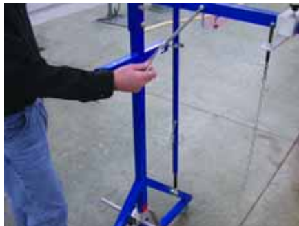
Adjust hex rod to obtain 92 inches from outside to outside of device.
