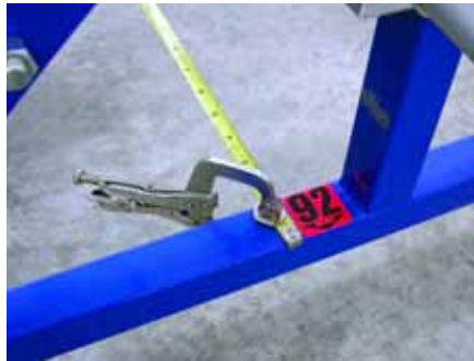
Clamp tape measure to outside of one side of device.
